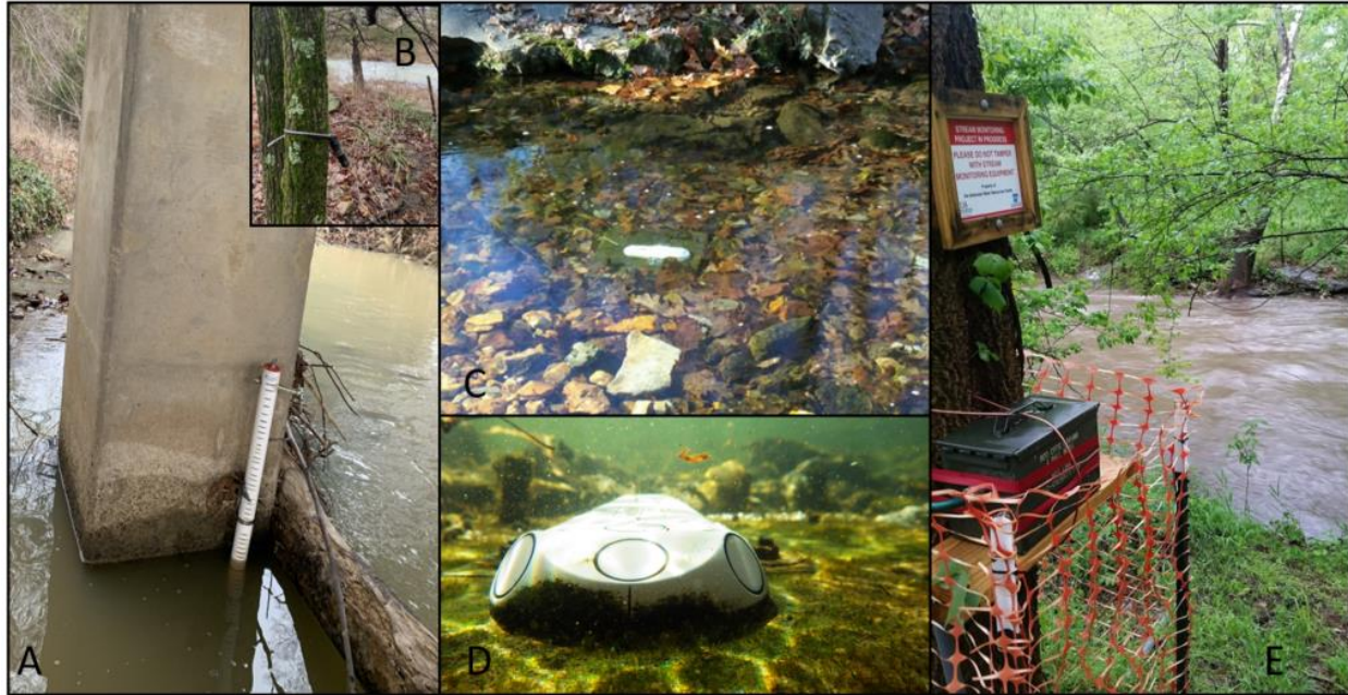
Figure 2: A) Pressure transducer installation on a bridge post, B) atmospheric pressure transducer attached to a tree outside of floodplain, C) SonTek-IQ attached to concrete block in stream channel, D) SonTek-IQ in stream channel, and E) ammo can attached to tree outside of the flood plain to store battery.
