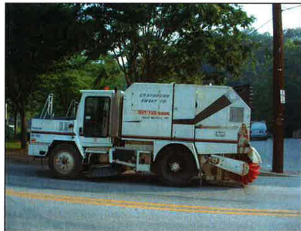
Figure 1. This broom sweeper is assisted by a following vacuum sweeper for increased removal.
